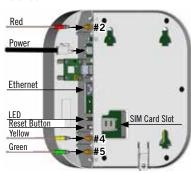
**Step 14** – Before connecting the power cable to the Gateway confirm that all connections are properly made. If so, connect the power cable. Turn the wall plate power switch to the ON position and verify that the LED on the backside
